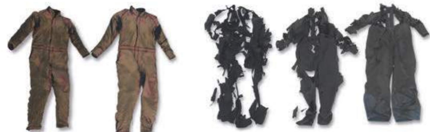
Nomex® Soft 183g/m² Nomex® Soft 203g/m² FR Cotton/PA 88/12% 237g/m² FR Cotton/PA 88/12% 305g/m² FR Cotton 100% 335g/m²
