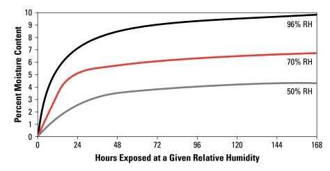
Figure 2 - MOISTURE ABSORPTION OF PRESSBOARD @ 50% RH AND 25°C
